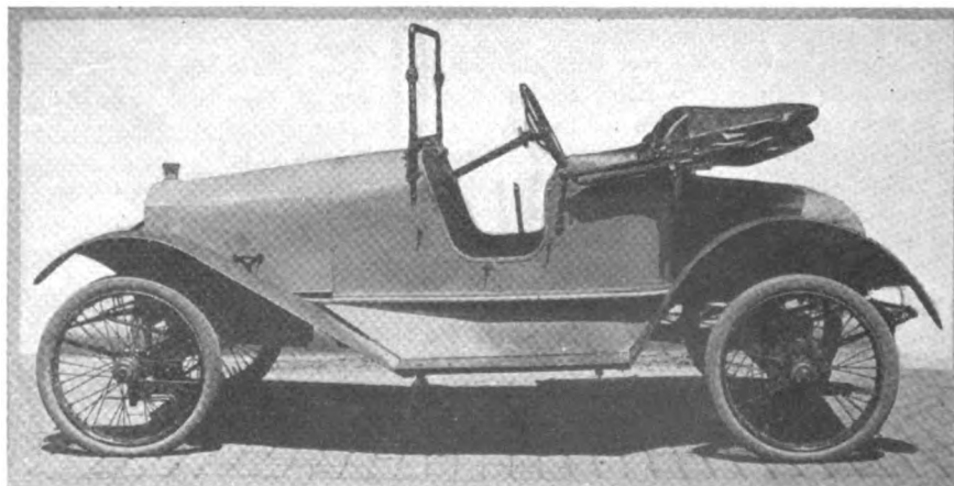
Side view of Argo, showing wire wheels, left drive and center control
